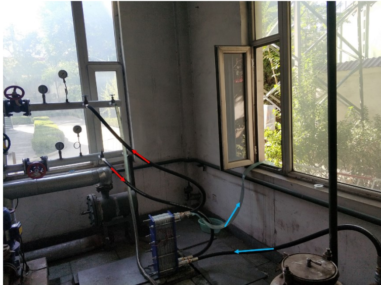
Figure 4: One of the TEG devices (20 layers) installed for field tests.
