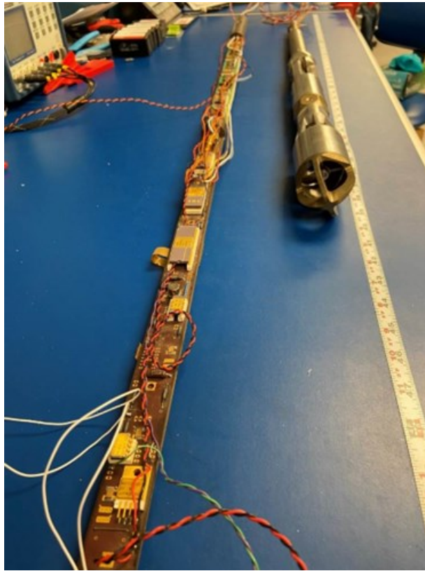
Figure 2: Sandia's custom high-temperature logging tool with Honeywell's microcontroller and Sandia's custom Application-specific Integrated Circuit or ASIC (left) next to Mitco's PTS module (right).
