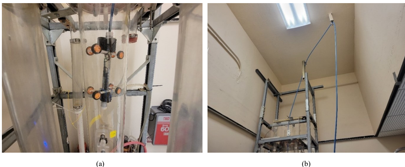
Figure 17: Modifications applied to the running mechanism to improve its operation: (a) updated driving mechanism, now using tool's electric cable to drive the movement in and out of the wellbore; (b) Updated routing of the electric cable connecting the chloride tool and the data acquisition (DAQ) hardware.
