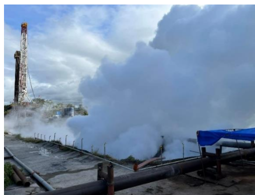
Figure 12: Simultaneous flow test of SPEC-B1 and drilling of SPEC-B4 at Well Pad P B
