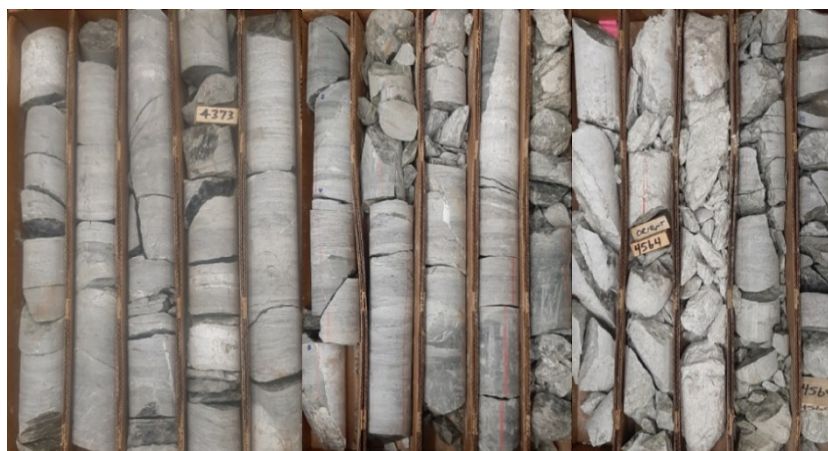
Figure A1: Core Images for Well A for 4373, 4470, and 4564 feet from left to right
