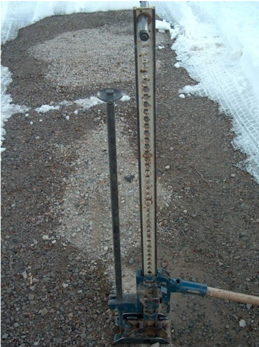
Figure 6. A 2' length of \frac{1}{2} " pipe slipped over a 2-meter probe to extend the range of pull after the height limit of the jack has been reached. Locking pliers can also be clamped at the base of the probe for additional pulling range or when the threaded end of the probe has been broken off, however the locking pliers can cut deep groves and leave sharp burs on a probe. Also note the "T" handle at the top of the jack column made from sections of \frac{1}{2} " pipe and a thru-bolt. This provides a grip for a second person to stabilize the jack when removing difficult probes. The person stabilizing the jack should be alert for pinch points when the jack running gear approaches the top.
