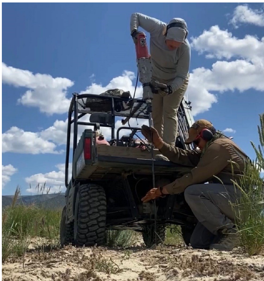
Figure 1: Example of GBCGE personnel driving a hollow steel probe into the ground using a demolition hammer.
