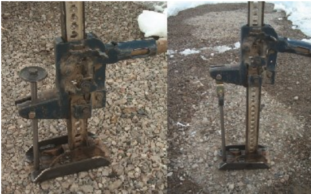
Figure 4. Standard methods of pulling a 2-meter probe showing the use of the hex nut welded to a washer (left) and (right) eye-nut linked to the jack toe. The heavy washer welded to the hex cap distributes the load on the jack toe to prevent marring of the slot in the toe and hex cap. Using the method on the left works well when the probe is far enough out of the ground to slip the slotted toe around the probe, or when the ground is soft enough to kick some dirt away to get the jack low enough to get the toe around the probe. Using the eye-nut, as seen on the right allows pulling probes with tops close to the ground without the need to dig a hole to get the jack toe around the probe. When screwing the hex cap or eye-nut onto the top of a 2-meter probe for pulling, screw the cap or eye on hand tight and then loosen it one eighth to a quarter turn. This allows easy removal of the thread stub if the threaded end of the probe should break when pulling.
