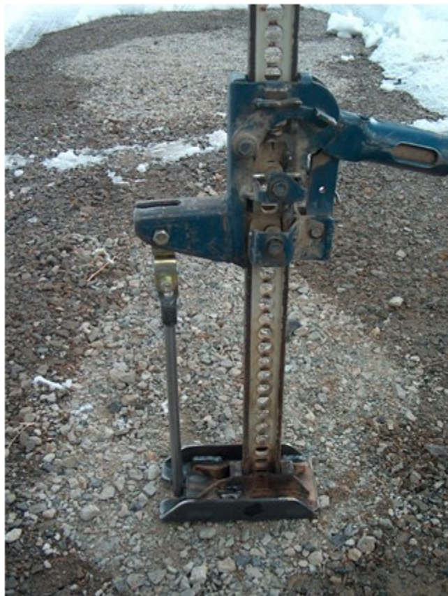
Figure 1. Pulling a probe with a threaded eye screwed to the top of a 2-meter probe using a modified jack.
