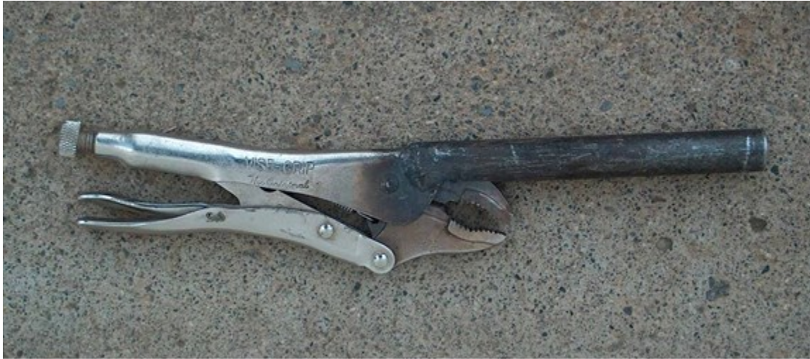
Figure 5. Locking pliers with ½” pipe extension welded to the fixed jaw. Some probes can easily be pulled out of the ground using these pliers.
