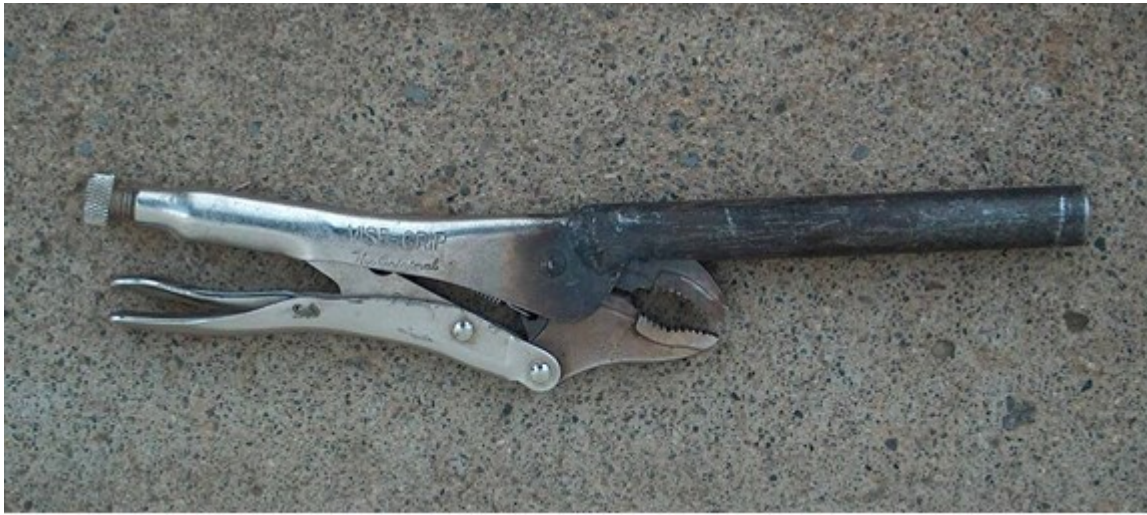
Figure 3. Locking pliers with 1/2" pipe extension welded to the fixed jaw. Some probes can easily be pulled out of the ground using these pliers.
