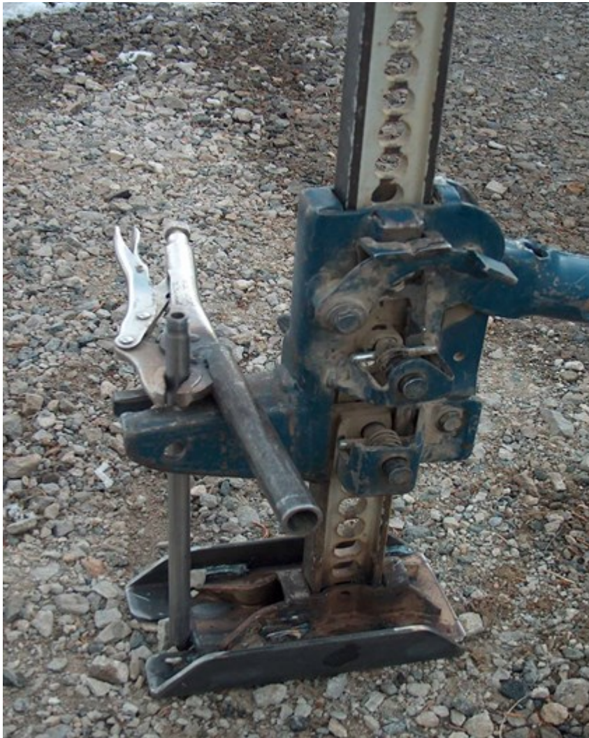
Figure 5. Using locking pliers to remove a probe with broken threads. A second set of pliers may sometimes be necessary when the pliers slip and gouge the probe. In some cases, it may be necessary to bend the probe over to prevent the locking pliers from slipping.
