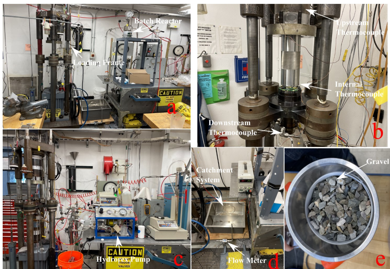
Figure 3: Photos of flow loop system equipment showing: a) the empty testing frame and batch reactor; b) gravel pack cylinder in testing frame; c) Hydrorex pressure system for maintaining constant flow through; d) flow meter and catchment tank for removing LCM that pass through gravel pack; e) untested gravel pack showing gravel and Teflon covering inside.
