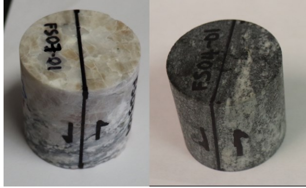
Figure 2: Subset of the Granite rock sample from Utah FORGE site, each with a diameter and length of 1.5 inches, cored to align foliation parallel to the direct shear plane for hydraulic and geomechanical characterization.
