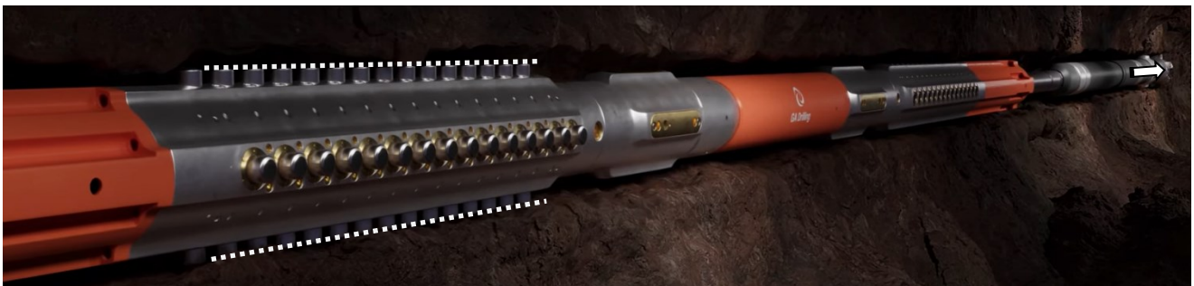
Figure 6,c) When Walking Section reaches the end of its stroke, the Upper Grippers extend during a hand-over period
