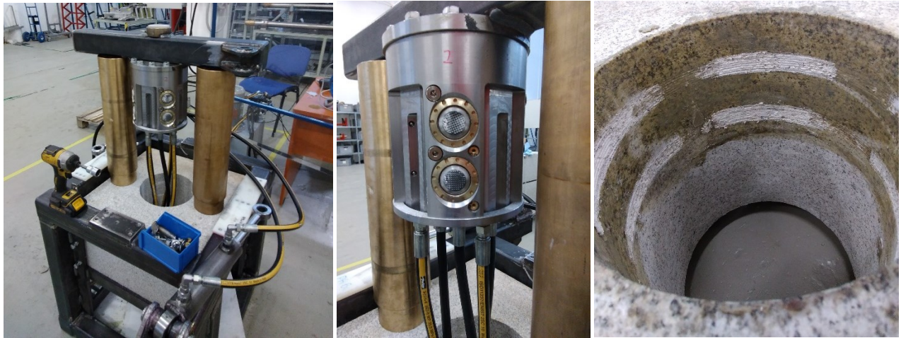
Figure 7 Test set-up of Scaled Prototype Test having eight grippers and applying continuously increasing torque (left and center); Granite sample after the testing with scratches caused by slip of the grippers after exceeding its torque capacity (right).
