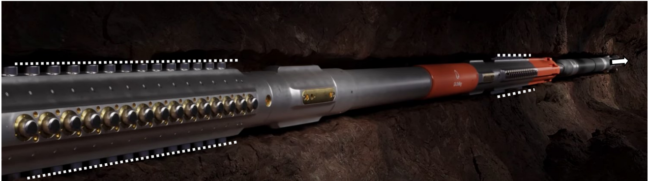
Figure 6, e) The process is now reversed, as the Walking Section extends, the Lower Grippers move downhole, faster than the bit.
