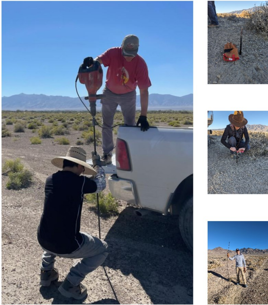
Figure 5. Shallow temperature survey probe installation (left and top right), Resistive temperature device insertion (middle right), and probe retrieval (bottom right).
