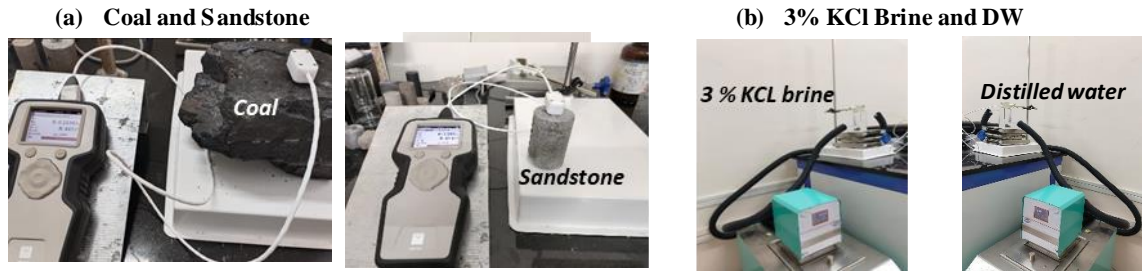
Figure 3: Experimental determination of thermal conductivity of rocks (sandstone, coal) and brines (distilled water, 3%KCl )
