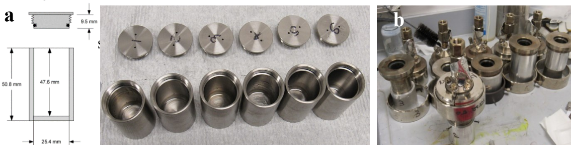
Figure 4: Equipment used for hydrothermal experiments involving produced microcapsules and sodium silicate solutions. To minimize fluid loss and chemical contamination of the samples, sealable internal cells (a) were used in combination with small Parr reactor vessels (b). These vessels were heated in a convection oven at 150-200 °C (From Nakagawa et al., 2023b).
