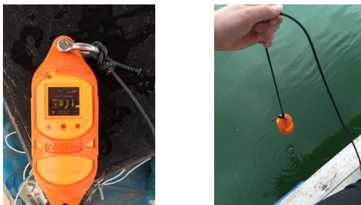
Figure 4: CTD logger with sensor for electrical conductivity, density, temperature, pressure and sonic velocity is lowered into the water on a rope.
