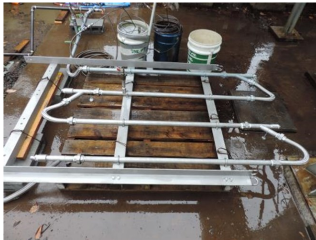
Figure 1: Corrosion test loop system at Kakkonda geothermal field
