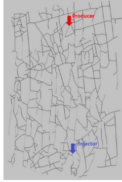
Figure 1 – Geothermal simulation model configuration with doublets position and Whitby fracture network configuration.
