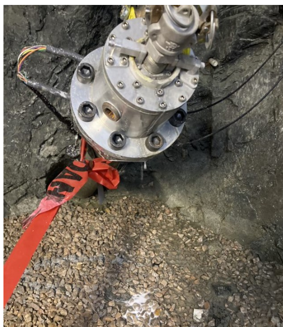
Figure 7: Milky fluid leaking from the AML collar observed on 17 August 2022.
