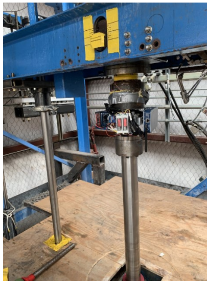
Figure 8: Photograph of the Bottom-Hole Assembly (BHA) emulator integrated with the Sandia HRDF.
