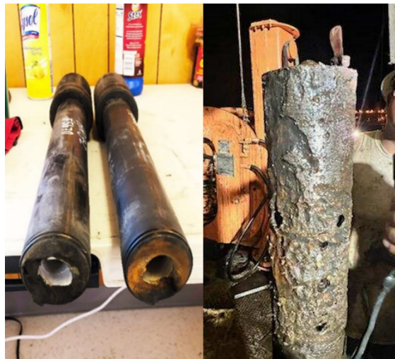
Figure 1. On the left: Two separate failures of the Acme Stub thread resulting in fishing operations. On the right: Corrosion on an 8-5/8 in. carbon steel hydroblasting head after approximately six months at 6800 ft from well A.
