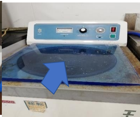
Centrifugal to precipitate clay
