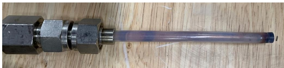
Figure 4: Ion-selective electrode configured for autoclave testing.
