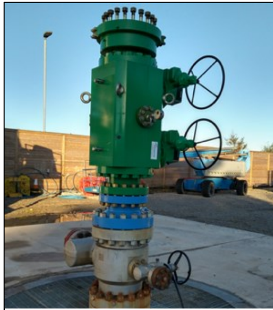
Hartmann master valve prior to testing
