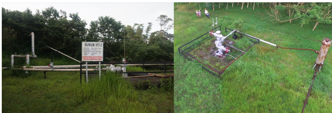
Figure 7. Declined wells in East Nusa Tenggara. Those wells are not connected to the production facility anymore, and just being bled to prevent gas accumulation.
