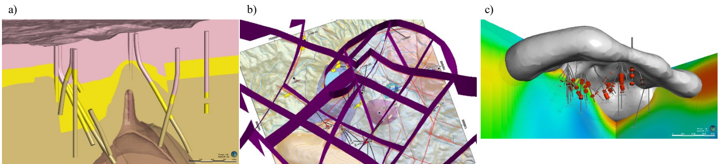
Figure 4: (a) A cut-away cross-section of the new Leapfrog geological model. (b) The new structural model shown above a map of the LGF. (c) The interpreted clay-cap viewed from below (grey) shown with MT resistivity slices and production wells with feedzones shown in red.
