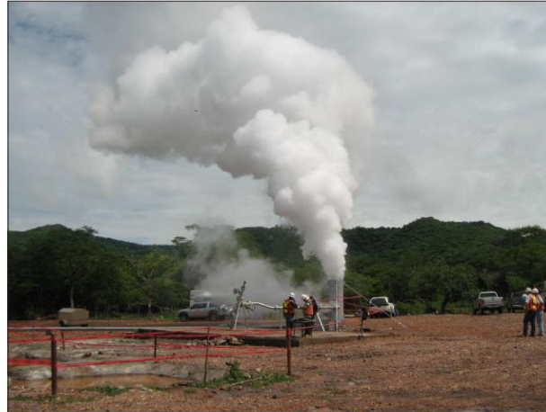
Figure 9: Discharge Testing Slimhole well MG-04 (White, P., et.al, 2010)
