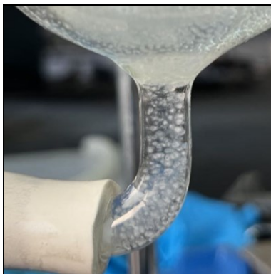
Figure 5: SAP crystal particles settling at the bottom of the tube
