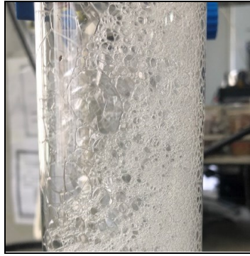
Figure 4: Foam with liquid holding rate of 18.9%
