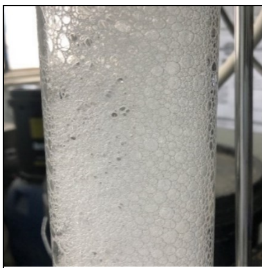
Figure 2: Foam with high water content
