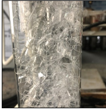
Figure 3: Foam with low water content
