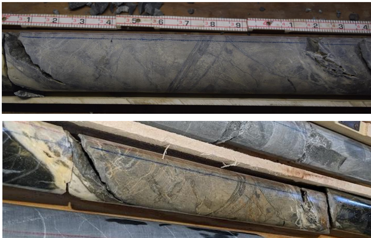
Figure 4. Core photo of E2-AML at ~187 feet deep, showing some open portions of a highly fractured interval.
