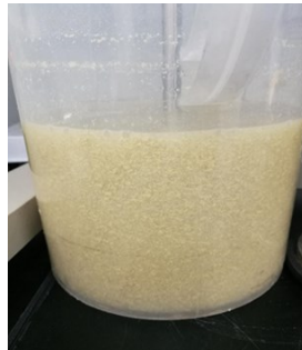
Fig. 10. Mixture of diverter and PAM solution
