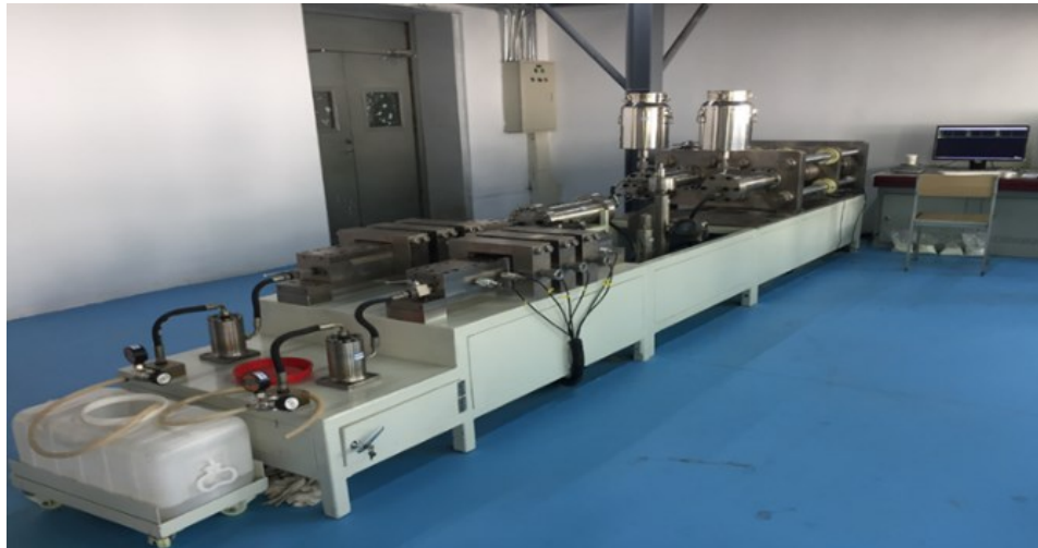
Fig.8. Experimental device for evaluating plugging performance
