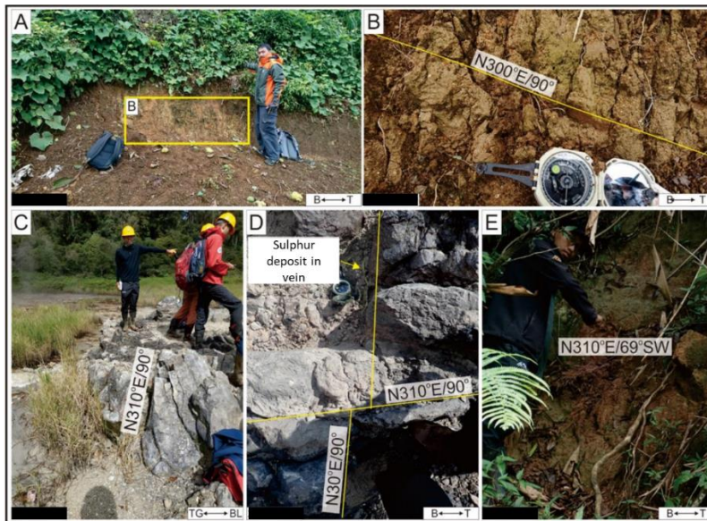
Figure 6: The fault measurement; (A) and (B) are the Babakan fault at the outcrop of pyroclastic lithology, (C) and (D) are the NW-SE and NE-SW faults at the outcrop of Andesite lava, (E) is the discontinuity surface at the slope of Mt, Urug, interpreted as the fault plane which triggers soil moved.
