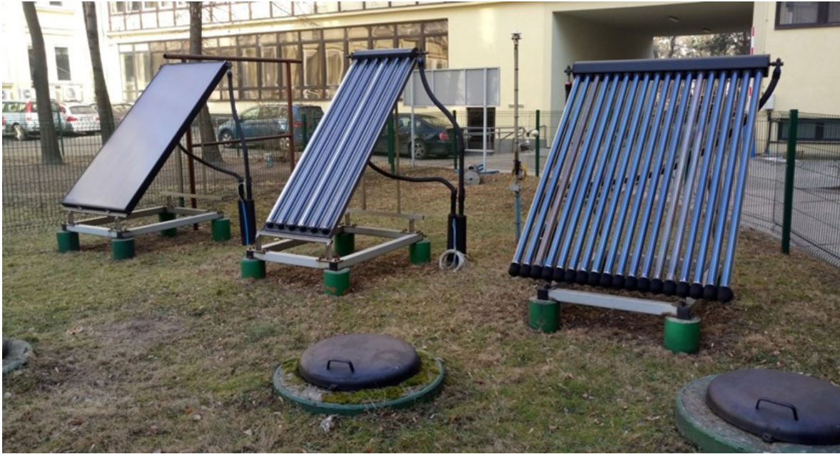
Figure 6: Solar collectors at the field station (Field A) and manhole flaps of BHEs in front of them.
