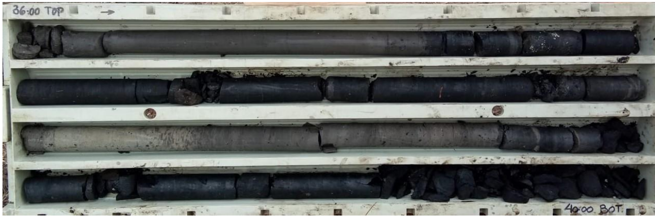
Figure 1. Core sample extracted by full core drilling operation during coal exploration in Kuala Kuayan
