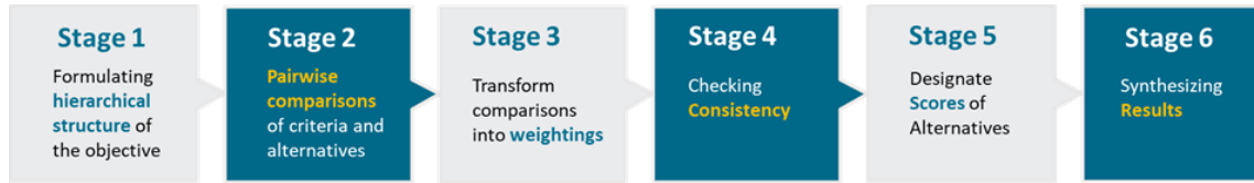
Figure 1. General framework of the AHP method (Raith, 2020)
