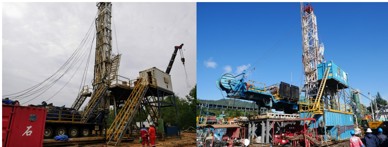
Figure 2. Example of smaller truck-mounted rotary drilling rig (350-750 HP)
