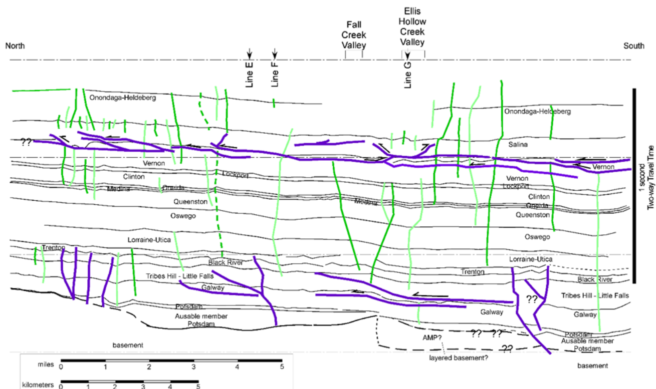
Figure 5 – Geologic structures interpreted from hydrocarbon industry 2D seismic line collected a few km east of the proposed Cornell ESH well site. Image is vertically exaggerated ~3.3 X. Purple = faults; Light green = synclines; Dark green = anticlines (Jordan, 2019)
