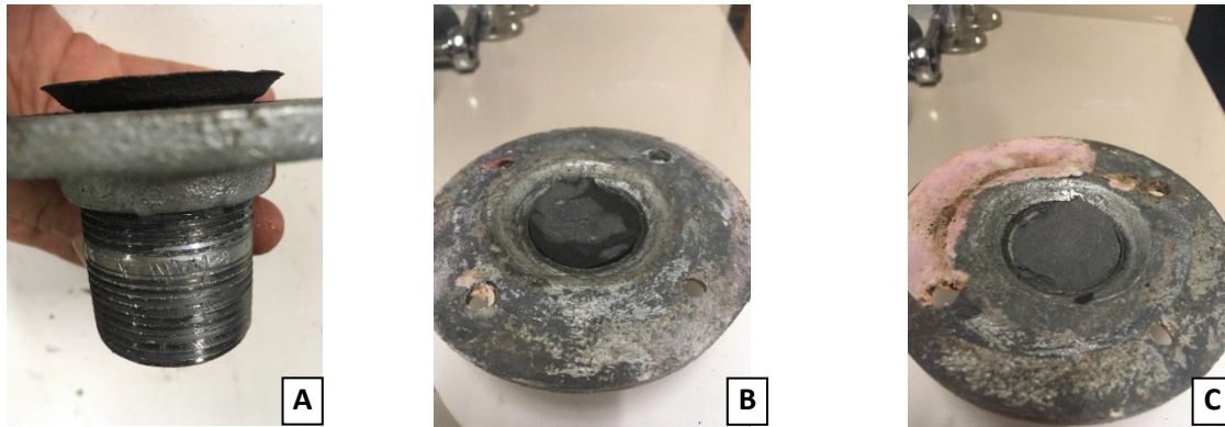
Figure 4. Shear bonding strength cell before testing (B, C) and after testing (A)
