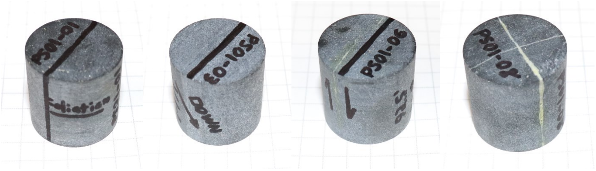
Figure 1: Subset of the prepared Poorman's schist specimens having 25.4 mm nominal diameter and cored to position natural fractures parallel with the plane of direct shear for hydraulic and geomechanical characterization.
