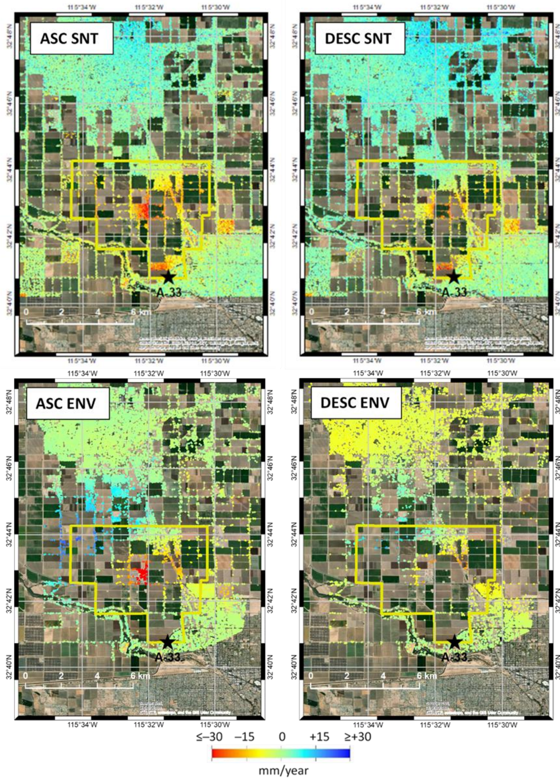
Figure 5. Maps of ascending (left) and descending (right) LOS rates obtained from the Sentinel (top) and Envisat (bottom) images.
