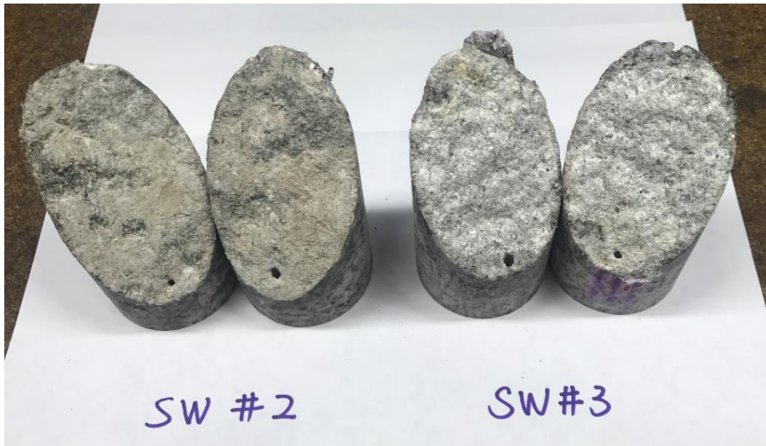
Figure 11: Gouge production and slickensides on tested samples SW #2 and SW #3.
