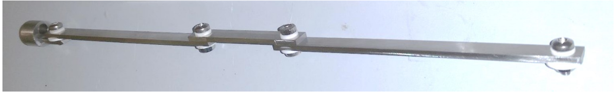
Figure 2: Corrosion samples assembled for testing. Three samples were in each test in the reactor.
