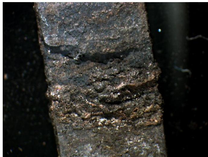
Figure 6: Crack on the surface of UNS N06625 sample
