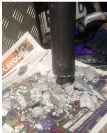
Figure 6. Calcite scale material recovered from the well (bailer tool diameter: 1.5”)
