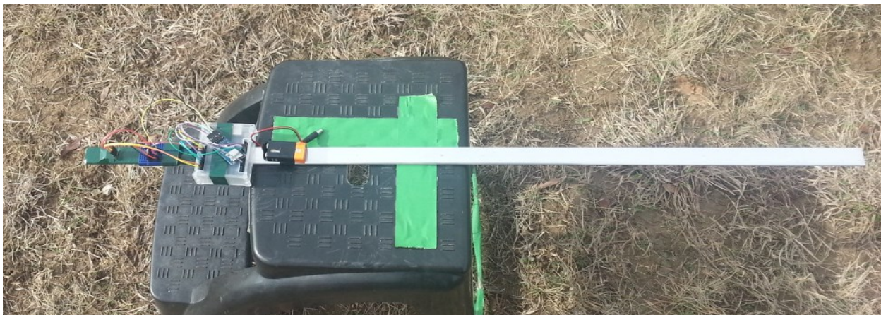
Figure 4 A simple exercise in programming an Arduino to measure orientation using three shields and a 9V battery.
