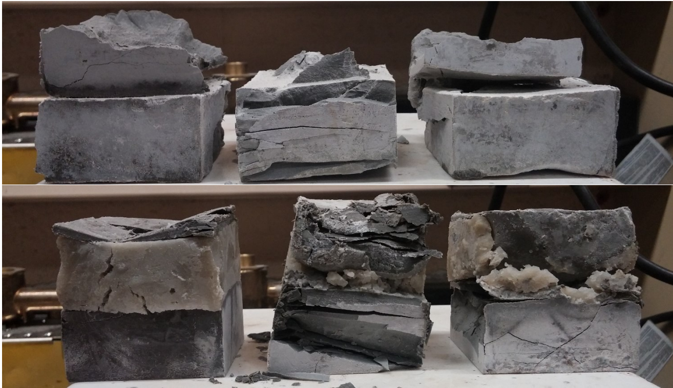
Figure 9 – Cube samples – top poured in annular water, bottom poured in drilling fluid, left samples kept at surface conditions, the other two samples exposed to 20°-90°C over 2 hours
