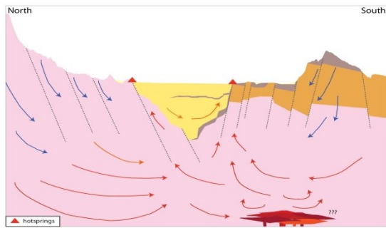
Figure 11) Cartoon illustrating our conceptual model of the structure and geothermal system of the Camas Prairie study areas.
