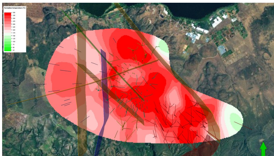
Figure 8: Horizontal view of the temperature distribution at -400 m a.s.l. (~2400 m depth) in the revised temperature model of the Olkaria geothermal system. Also shown are the main faults/fractures of the system.
