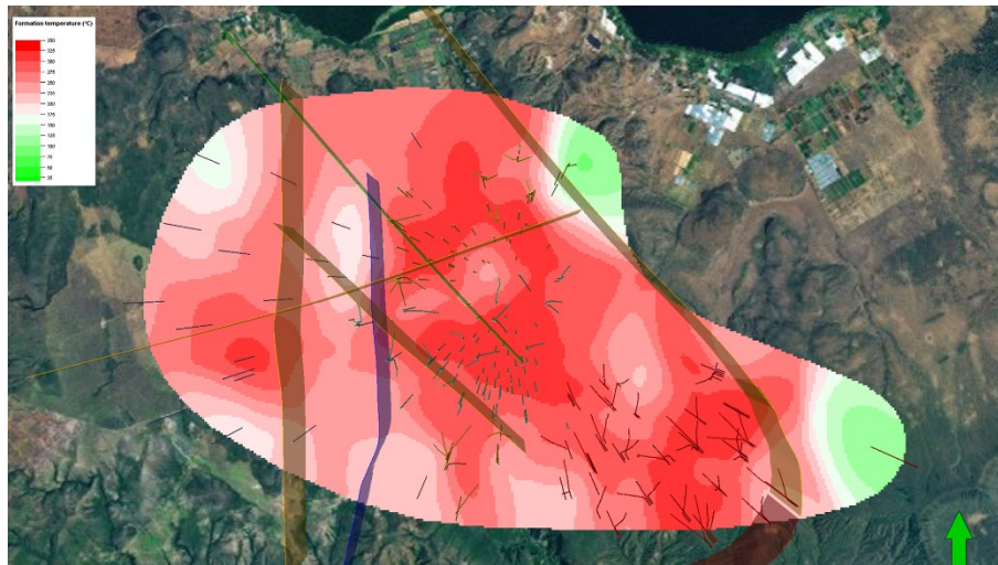
Figure 6: Horizontal view of the temperature distribution at 400 m a.s.l. (~1600 m depth) in the revised temperature model of the Olkaria geothermal system. Also shown are the main faults/fractures of the system.
