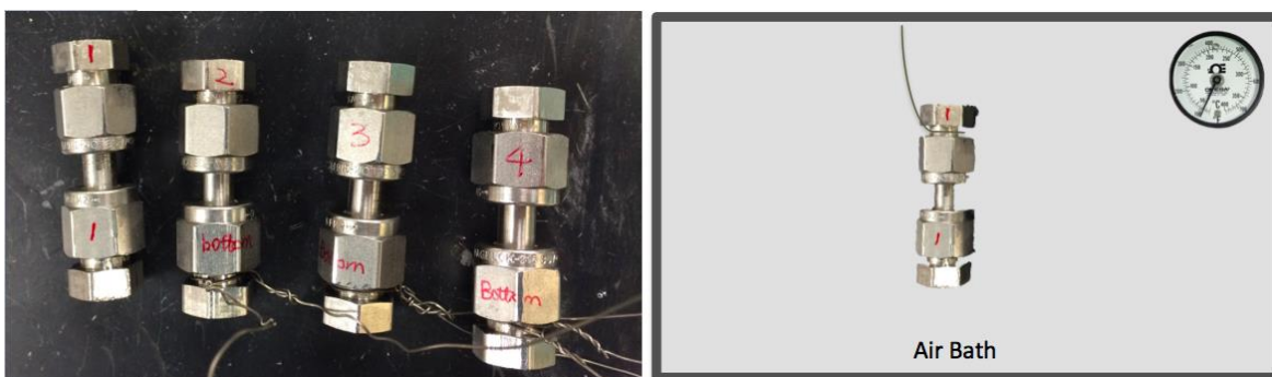
Figure 7: Schematic showing the vessels that contained DNA-silica nanoparticles during heating experiment (left) and how heating was conducted (right).
