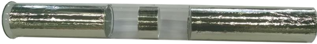
Fig. 10: Inner pipe of the glass Dewar flask with wrapped MLI
