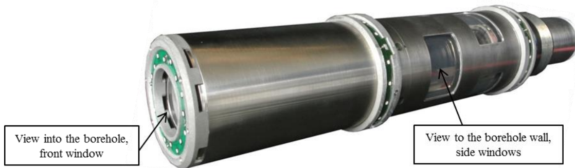
Fig. 6: Housing of the camera module; several windows allow a detailed axial and radial view to the borehole [Spatafora 2015-a]
