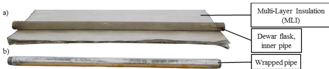
Fig. 8: Thermal insulation of the GeoKam inner pipe of the steel Dewar flask with wrapped MLI
