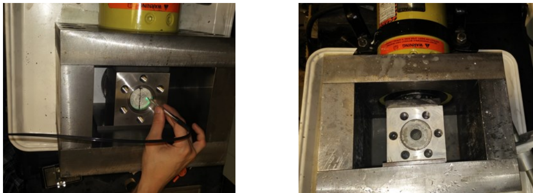
Figure 6: Measurements being performed after one week of curing (left) and sample with 19 mm hole drilled in center of core to produce stress concentration (right)
