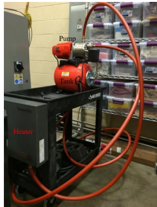
Figure 2: Hot water circulation system.
