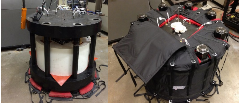
Figure 1: Polyaxial frame with insulation foam (red) and the Faraday cage jacket (black).
