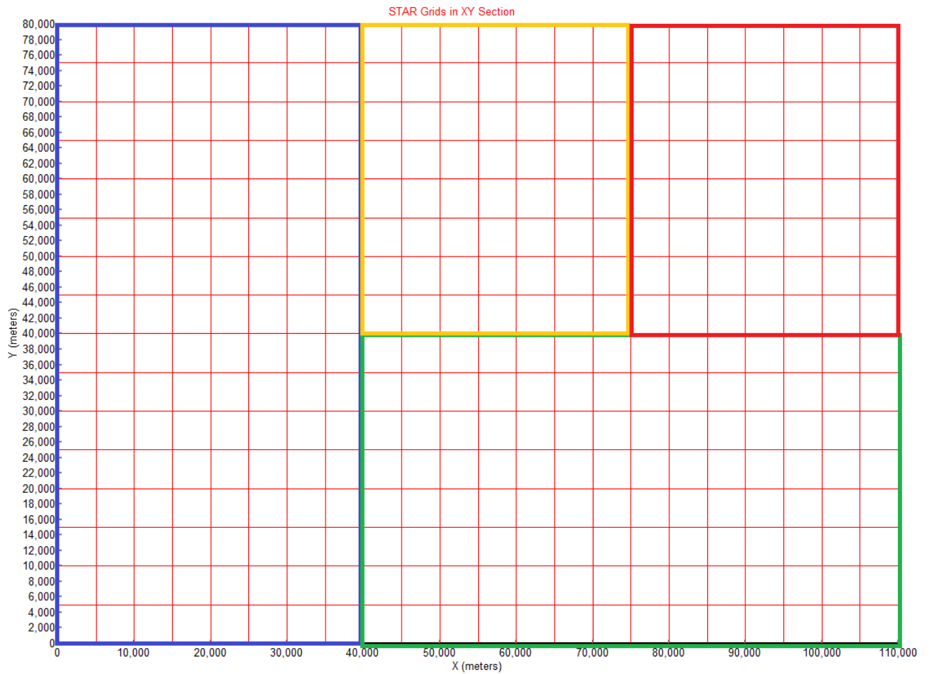
Figure 4: Heat flux distribution along the bottom boundary. Area enclosed by 1. blue outline, heat flux = 60 mW/m 2 , 2. green outline, heat flux = 75 mW/m 2 , 3. yellow outline, heat flux = 100 mW/m 2 , and 4. Red outline, heat flux = 110 mW/m 2 .
