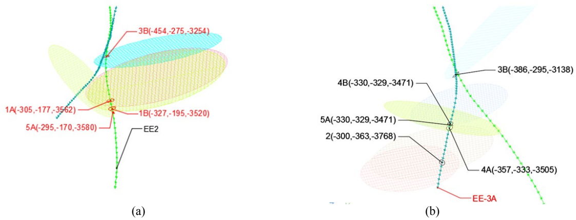
Figure 5. Location of the fracture-well intersections of the fractures with borehole EE-2, (a); and with borehole EE-3A, (b).
