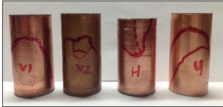
Figure 13: Pictures of samples after testing; copper jacket hasn't been removed to prevent sample disintegration. Red lines show clear fractures seen on surface. Location of these fractures in 3-D has been studied in next section using acoustic emissions.
