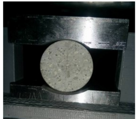
Figure 14: Axial force vs time plot for sample B1 (left) and picture showing the crack at centre of sample after Brazilian test.
