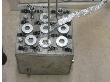
Figure 13: Instrumented medium strength concrete sample block used for concept validation testing.
