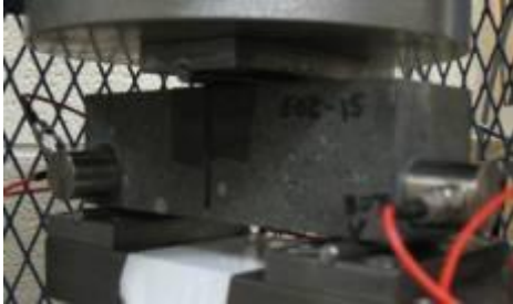
Figure 5: Image of the notched beam fracture test being performed on a short beam sample with a three-point loading configuration.
