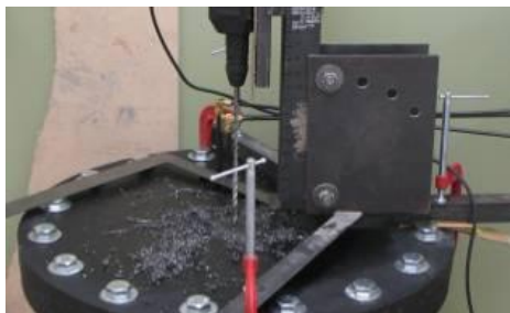
Figure 2: Loaded cell with borehole being drilled using the oriented drilling rig.
