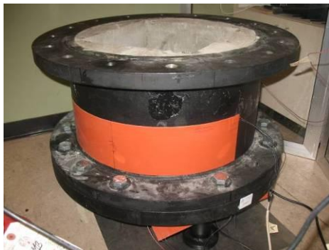
Figure 1: Unloaded heated true-triaxial load cell.
