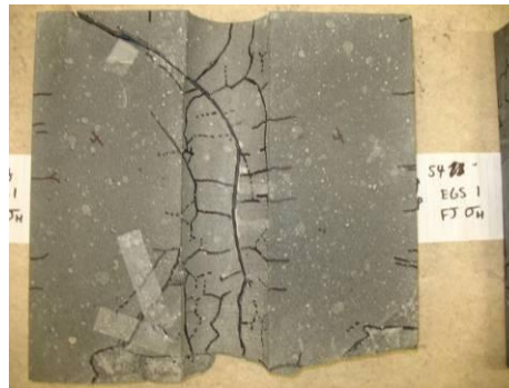
Figure 10: Cross-section of the sample fractured during the systems integration test. The observed fracture traces are marked with black ink for better visibility.
