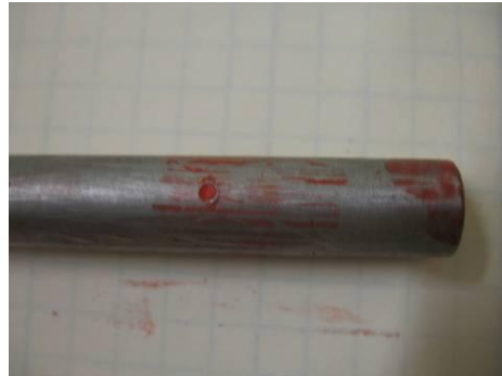
Figure 7: Image of the perforated borehole casing used for the systems integration test with wax plugged perforations.
